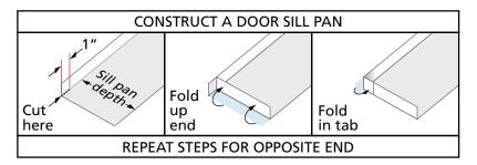
J. If there is a step down at the exterior of the door opening, cut the sill nosing to the rough opening width plus two times the flange width. Notch the sill nosing. If there is NO step down, skip to step K.
